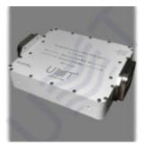
The repeater block is used for weak X-band RF signals amplifying from two antennas. The gain is carried out by two blocks of amplifiers and bandpass filters. X-band repeater block is applied in GSM / MVDS / MITRIS systems
