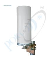
Ku-band OMNI slotted waveguide antenna is designed for MVDS/MMDS broadcasting systems at Ku-band range. It has 360 deg pattern, 1 GHz bandwidth and high Gain 12 dBi.
