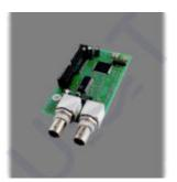
DVB ASI TS output board is designed to convert the parallel DVB TS into ASI TS and can be used with other our boards for building IP-ASI converters, receivers and other digital broadcasting equipment.
