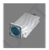
Ku-band LNB PLL LO 9.75 is Low Noise Block Down Converter with single LO 9.75 GHz and single 75 Ohm F-type output. LO instability: ± 150 kHz, Gain: 45 dB, Noise figure: 0.9 dB, Output power P1dB: +3 dBm.
