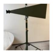
Directional 5.8 GHz Wi-Fi horn sector antenna (HORN55\_750R) with 24 dB gain, circular polarization, and SMA female connector. Designed for UAV video channels, it offers <1.5 VSWR, 11° horizontal beamwidth, and robust aluminum housing.
