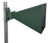
This 5.8 GHz Wi-Fi Horn Sector Antenna offers a strong 19 dB gain and optimized directional beam pattern, making it ideal for reliable point-to-point or sector communication. Designed for telecom professionals and RF engineers, the antenna features a durable build, SMA connector, and excellent VSWR performance. Whether for drone video links or long-range Wi-Fi networks, this horn antenna ensures stable, high-quality data transmission.
