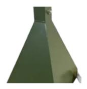
High-performance 2.4 GHz horn sector antenna with dual RHCP and LHCP circular polarization.
